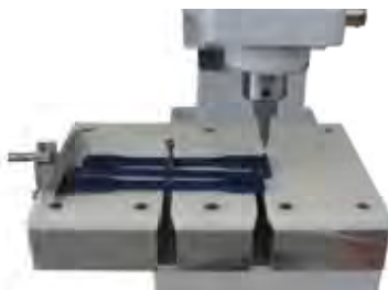
Specimen punching machine / Gate- and runner cutting
