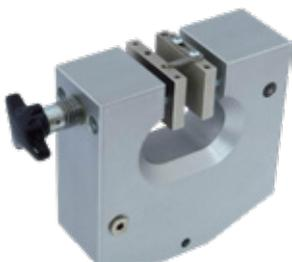
Pneum. Spannzeug, Spannkraft 7 kN, Klemmfläche 40x60 (100) mm
