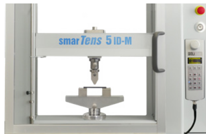
3-Point bendig fixture mounted on a 5 kN smarTens UTM
