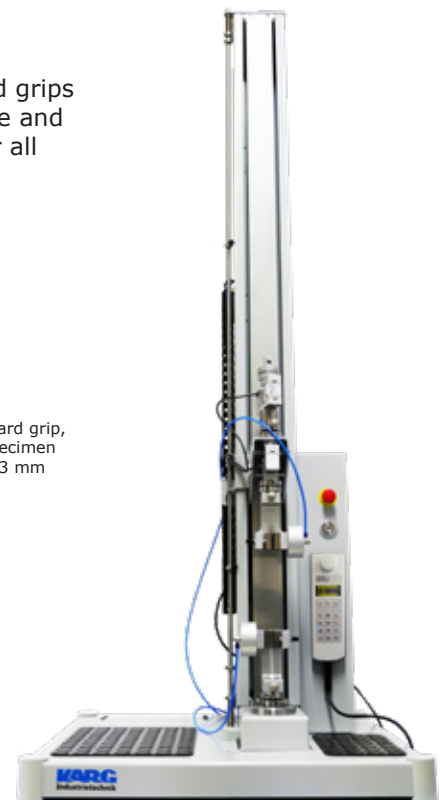
smarTens 2.5 IS-L with pneum. grips for film testing
